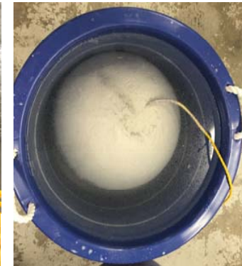
4. Cure the concrete in water for 14 days
